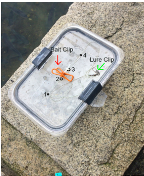
Figure 2. One of the “bait boxes” used in the study. Magnets or rocks (control) were covered with tin foil and placed in the box. Bait was placed on top of the box in the bait clip. The box was lowered into the water by attaching fishing line to the lure clip.
